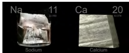
Fig.2 – Metals frequently added to EHC fluids from acid filters
