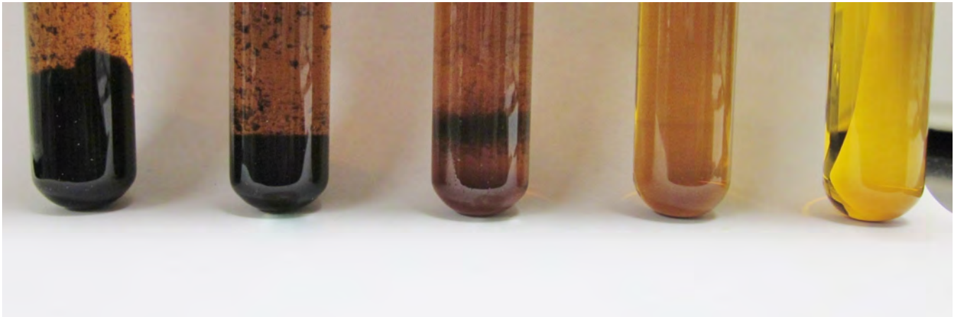
Fig. 10 —In Step 1 of the Deposition Tendency Test referred to in the EPRI EHC Fluid Maintenance Guide 2002, Page 4-39, EHC fluid is mixed with Hexane which forces out dissolved contamination into solid form. In the first three test tubes, EHC fluid using conventional treatment form visible solids. Servo-valve performance and reliability
