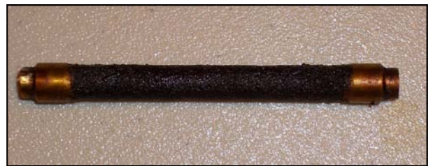
Servo pencil filter plugged by varnish
