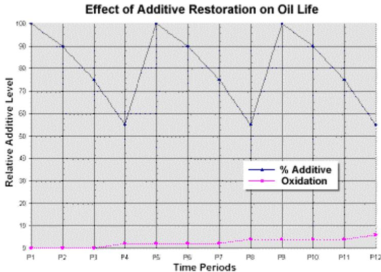
The additives start the next cycle from a very high level and the same scenario takes place. Again a very small amount of oxidation takes place. The oil is reclaimed again and the additives restored. **The net effect is that oxidation is controlled at very low levels, water and contaminants never build up to troublesome levels, Oil Life can be extended MANY TIMES!**
