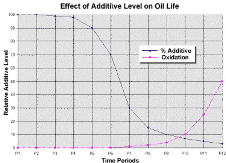
Eventually the degree of oxidation will reach the point where the lubricant must be removed and replaced with new oil. Reclamation at this point is not recommended.
